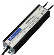
FSP150-FZAE(070) VG V Type: IP67 rated with 1-10V Dimming Function M Type: IP67 rated with 1-10V, PWM Dimming Function (only 2.8A/3.15A) Blank Type: IP67 rated and without Dimming Function R Type: IP65 rated and output current can be adjusted through internal potentionmeter
