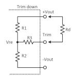
$$Ru = \frac{aR_2}{R_2 - a} - R_3 \quad a = \frac{V_{ref}}{V'_o - V_{ref}} \cdot R_1$$
